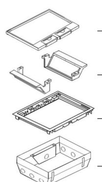
Floor Box cover w/ recessed space for the floor covering material. (7/16" max.) (Supplied)
